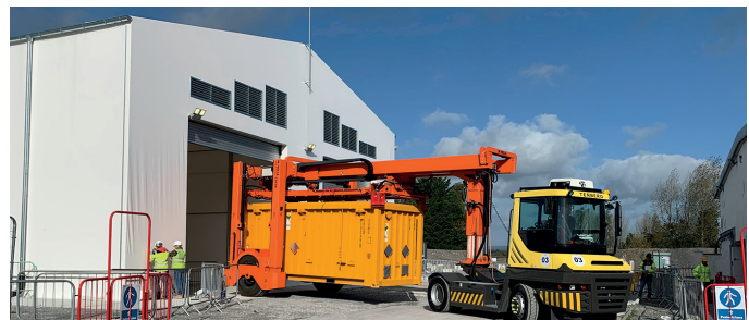
A 'Movella' container mover transports the empty and full containers between the container laydown area and the enclosures.
