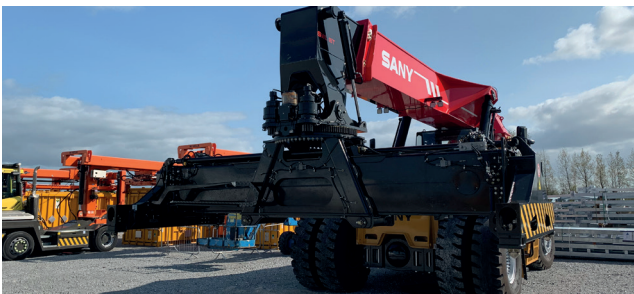
Container reach stacker this is used to lift the containers on and off the trailers and stack them in the container laydown area.
