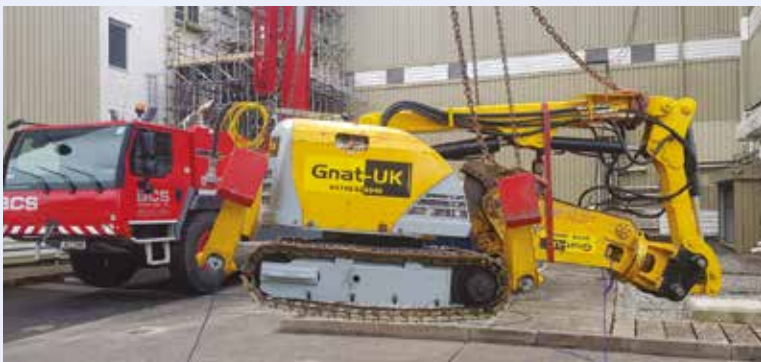
Machinery used during the 'Clean to Shell' and 'Demolition' phases - Brokk demolition robot used to remove equipment from buildings (left) and high-reach machine being used during demolition (right).
